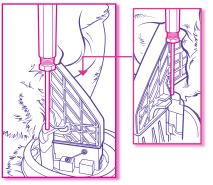
Fasten 2 screws onto the top of the head-turning mechanism.
