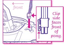
Snap in electrical connector clip from head into body. Make sure clip side of connector faces toward front of pony.
